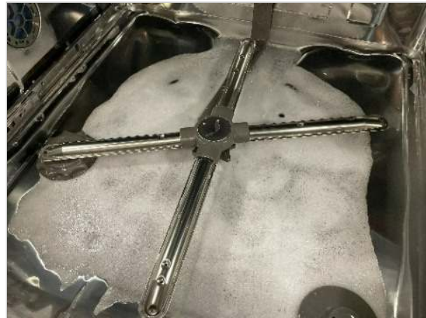
Unit not draining properly.
